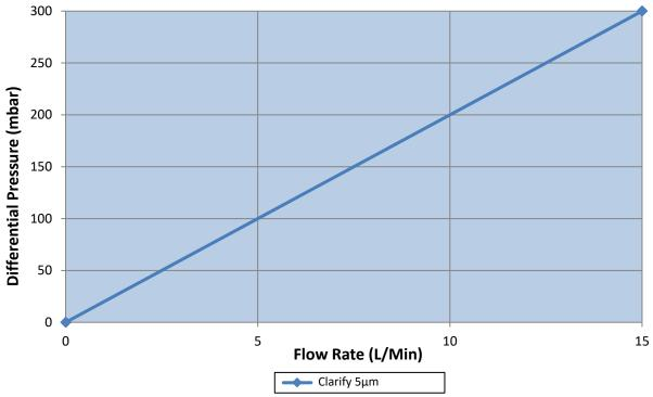
Speeds per 10" cartridge length filtering air at 20°C/68°F. Typical pressure drop values obtained from the tests, with the housing pressure drop deducted, are shown below:
